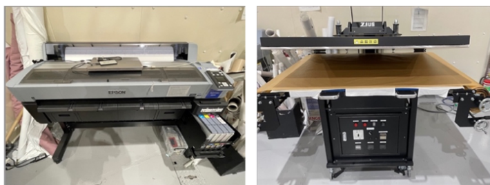
Figure 4: Inkjet printer for sublimation transfer (left) and thermal transfer device (right).
