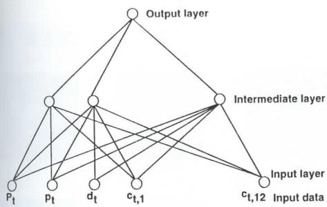
Fig.4 Configuration of a sub-network
