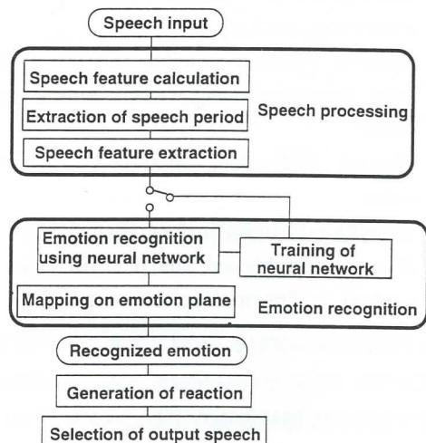
Fig.1 Blockdiagram of the prcessing flow
