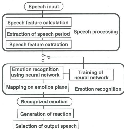
Fig. 1 Blockdiagram of the prcessing flow
