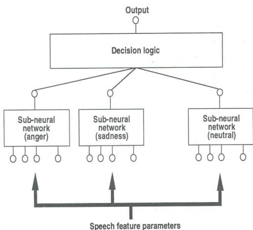
**Fig. 3 Configuration of emotion recognition part**
